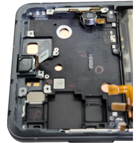
Vibrator Motor Disassembly Point
