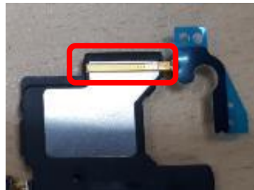
Attach an ANT-FPCB to Speaker-R
