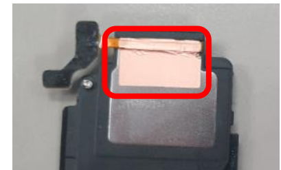
Attach a CU Tape to Speaker-L
