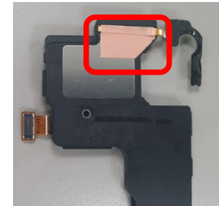
Attach a CU Tape to Speaker-R
