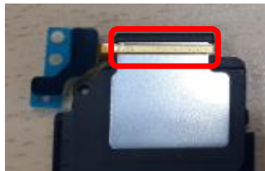
Attach an ANT-FPCB to Speaker-L
